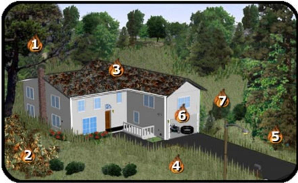
**1) Remove dead or overhanging branches.** During the windy conditions that exist during a wildland fire, flames, sparks and firebrands could travel from the tree to the roof of this structure.
